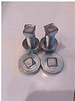
Figure 1. Break surface of coach bolt (article number 90002944) – bolt head separated from bolt rod
