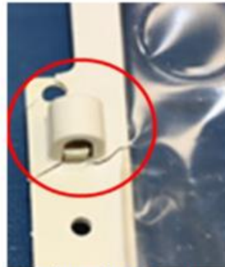
Membrane Frame Breakage
