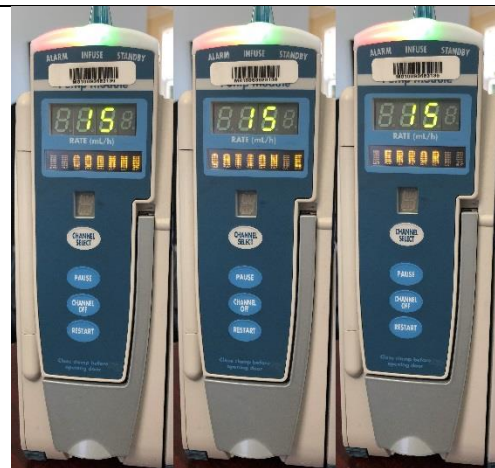
Figure 2: COMMUNICATION ERROR message on the module
