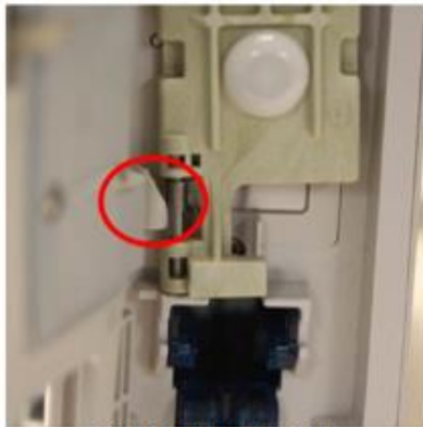
Broken Platen Lower Hinge Bracket
