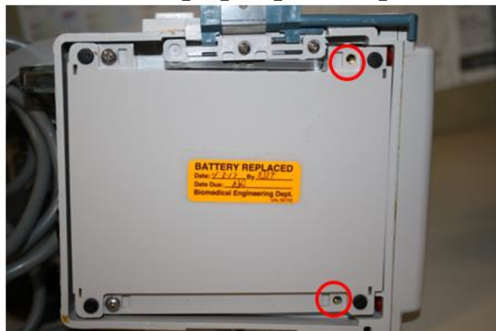
Figure 5: Bottom of Alaris™ PC unit highlighting 2 missing screws and washers
