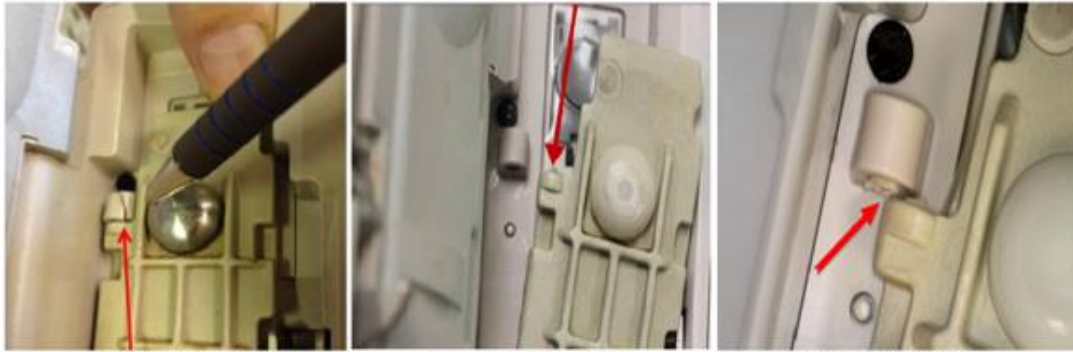
Cracked Hinge on Membrane Frame
